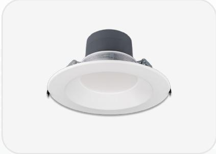
Our high-brightness commercial downlights feature 5 selectable wattages and 5 CCT options, delivering flexible, efficient lighting. With up to 2750 lumens, 90+ CRI,  $\geq 114$  lm/W max efficacy, and smooth 0–10V on 120–347V, they provide reliable, high-quality illumination for residential and commercial applications.
