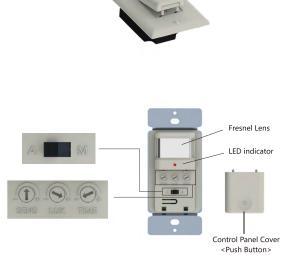
Remove the cover below the sensor lens by inserting a small screwdriver into the notch on the bottom of the cover.
