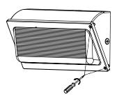
1. Loosen the two M5 screws.
