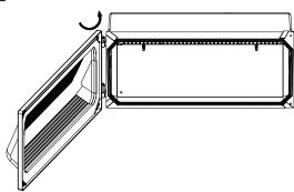
5. Reinstall the glass cover frame. REMOVE THE WATERPROOF PLUGS.
