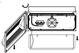
2. Remove the glass cover & the reflector.
