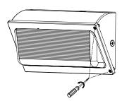
6. Tighten evenly back the two M5 screws and check whether the fixture works properly.
