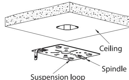
Step 3: Connect the clip from the fixture to the spindle of the mounting plate to make sure the fixture will not slip and fall. Connect the line voltage to the wires coming out from the fixture as shown in the wiring diagram. Push the pressing plate into the suspension loop on the mounting plate.
