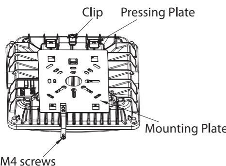
Step 2: Fix the mounting plate to the ceiling with the screws.
